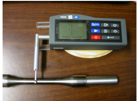
Sample application of 90° extension
