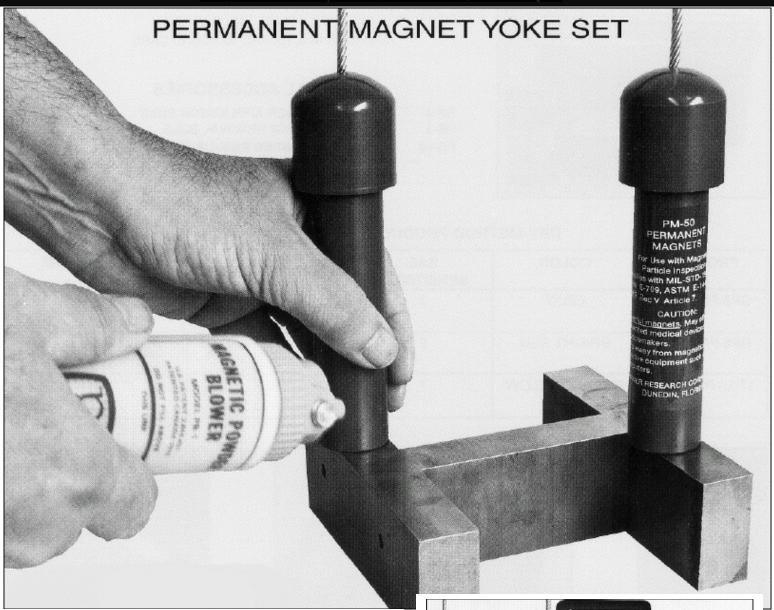
For Magnetic Particle Inspection applications (where applicable) per specification: ASTM E 709, ASTM E 1444, ASME Section V Article 7 and MIL-STD-1949. Certification included.
