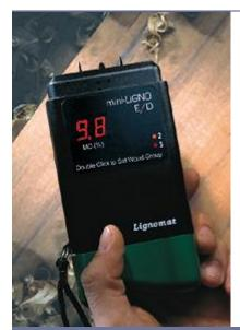
The mini-Ligno E/D moisture meter has a bright, easy-to-read, digital display and a wide moisture range - at an affordable price. Great for occasional use or in-line measurements. The moisture range is low enough for cabinet makers, professional woodworkers and hardwood floor installers and high enough for construction lumber, wood turning, pallet making, forest fire prevention and testing of firewood.
