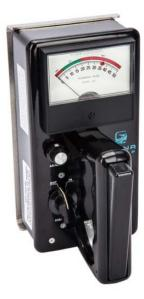
This instrument is similar to the LG instrument, except that it has a stainless steel flat plate electrode. Excellent for testing Gypsum Wallboard as it moves or in stacks. Measures the moisture in the Gypsum plasterboard 1/4 inch to 3/4 inch thick. Color Coded direct reading dial for fast comparison. Can be used to check the moisture distribution pattern on the board-along the length or width. Complete with a Carrying Case, NiMH Battery and Operating Instructions Book.
