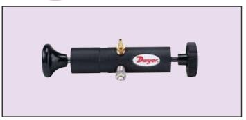
**Serves as pressure source** to calibrate gages and transmitters or to set pressure switches. Use with manometer or other pressure standard. Includes volume adjuster enabling fine pressure control and bleed valve. Generates pressures from a fraction of an inch w.c. to 72 psig (5 bar). Includes barbed fitting, tee connector and three 36 "lengths of vinyl tubing.
