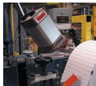
SG-300, Strobe Guard, Flex Arm SAS-DT-300, Flash Tubes and Sensors, shown in typical print inspection/ registration application.
